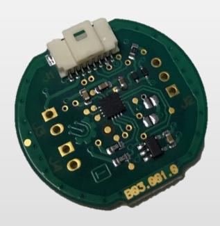
The **EM29** magnetic encoder, developed by Sangalli, has excellent resolution and accuracy at a very competitive price. The encoder provides absolute information both as single turn and multi-turn. The extremely small dimensions allow it to be used even on 40mm frame size motors (size 0). The communication protocol is the bi-directional Biss-C that allows the use of an electronic tag. The multi-turn position data is maintained even after switching off by use of a buffer battery.
