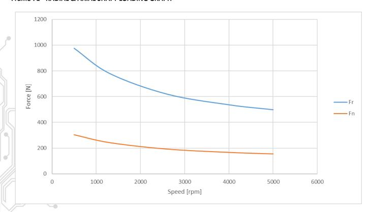
Frame 90 - RADIAL & AXIAL SHAFT LOADING GRAPH
