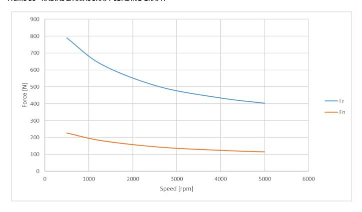
Frame 71 - RADIAL & AXIAL SHAFT LOADING GRAPH
